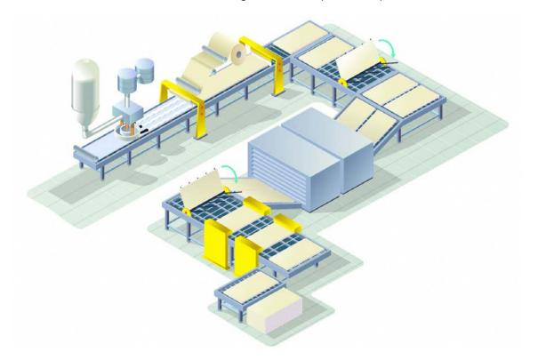
The initial materials are homogenously mixed to form a gypsum slurry that is spread via multiple hose outlets onto a glass fibre mat on a moving belt conveyor. A second glass fibre mat is fed onto the production line from above to form the glass reinforced board. The glass reinforced board continues along the production line where it is finished, dried, and cut to size.
